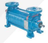
Side channel designs fill the hydraulic performance void between positive displacement pumps and centrifugal pumps. Fully open "star" impellers interact with the side channel casing creating an intense transfer of energy to the pumped liquid or liquid / gas mixture. The corresponding pressure increase (pump head) equals 5 to 10 times the amount generated by a similar size centrifugal pump at the same RPM.
